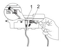
3. Place the power cord (1) in the right molded channel and the telephone cord (2) in the left molded channel on the bottom of the Base Unit.
